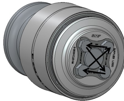
Correct sequence for tightening screws
