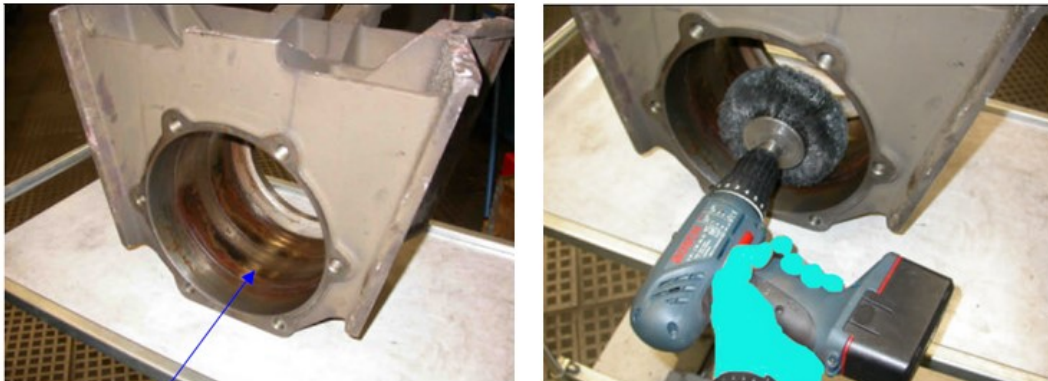
Removal of fretting corrosion
