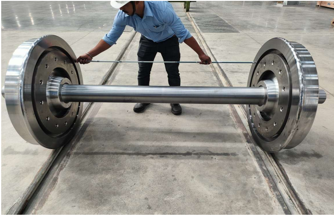
Measured with Mitutoyo make Stick Micrometer (137-204)
