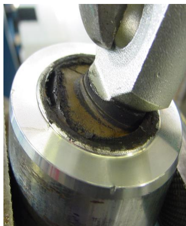
Figure 5-4; Examples of worn bushings
