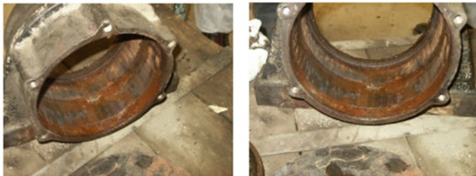
Fretting corrosion on an axlebox back from service
