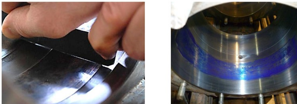
Inspection with ruler (left) and with contrast liquid (right)
