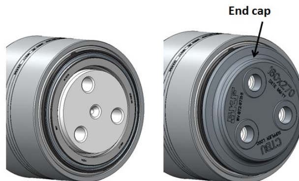
End cap assembling
