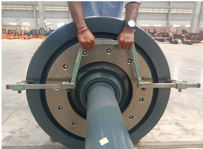
Wheel diameter gauge Paragon Instruments Engineers model "PIE WD-1(M)"
