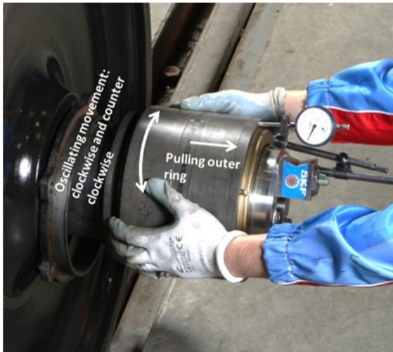
Movements to be applied to the outer ring to check the axial clearance correctly
