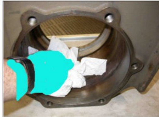
Wipe dry thoroughly all around the bore.
