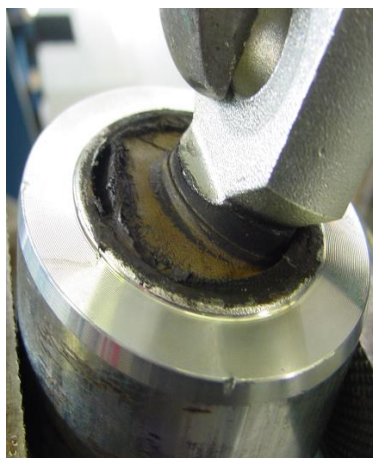
Figure 5-9; Examples of worn bushings
