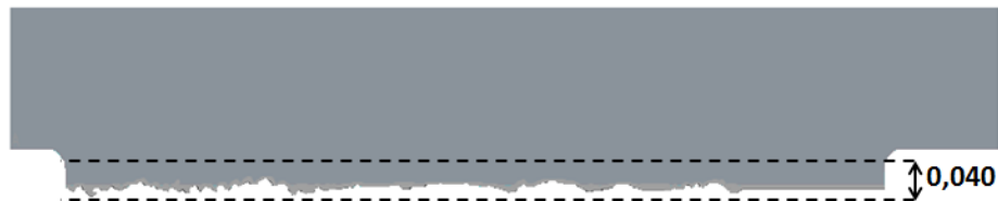
Example of a profile in the limits of cilindricity
