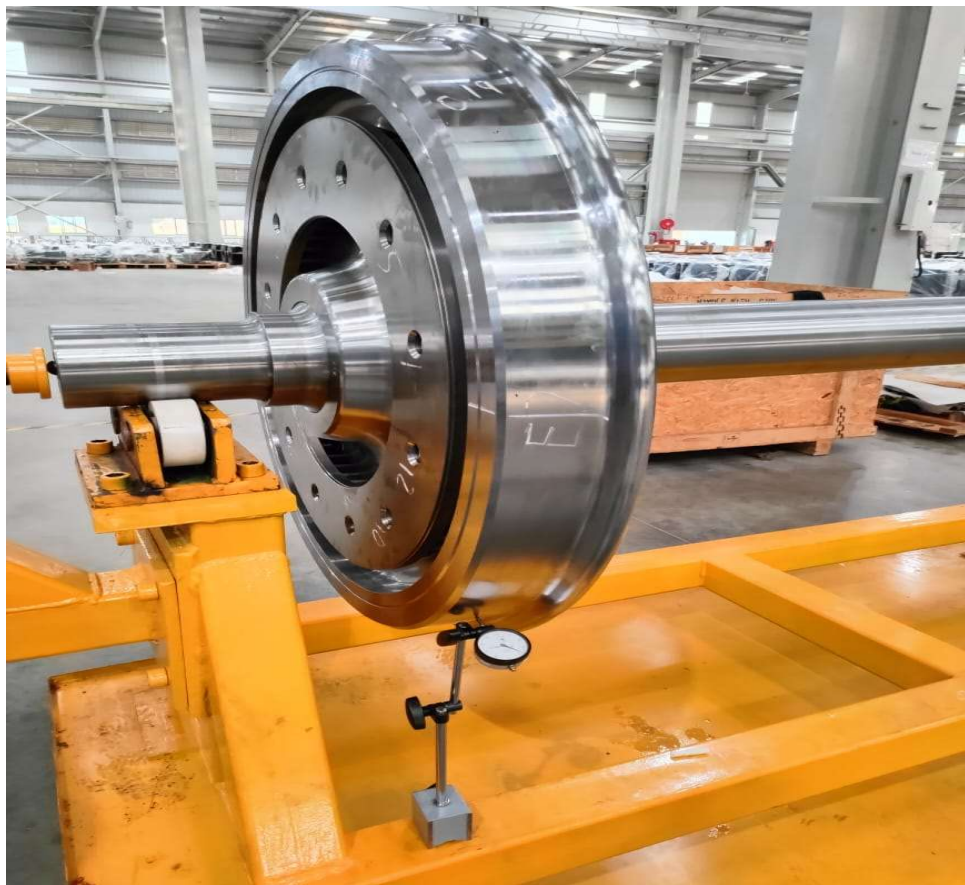
Measured with Mitutoyo Plunger Type Dial Gauge L.c-0.01mm range 0-10mm (2046A) with magnetic stand
