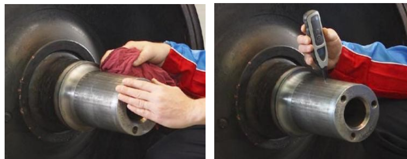
Cleaning and temperature measurement of the journal
