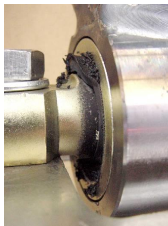
Figure 5-9; Examples of worn bushings
